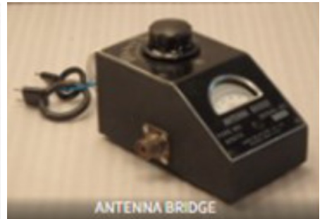
Millen Antenna Bridge
