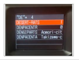
A list of rooms that match your criteria, in this case "D-E" appears. Using the knob, highlight the room you want to connect to and press the knob to connect to it.
