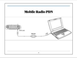
Another way to get to Wires-X is by connecting any of these mobiles to a computer connected to the internet with a separately purchased cable. Using a Portable Digital Node, you can access rooms and nodes from around the world any time you like, for as long as you like.
