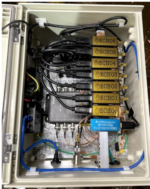
ECHO RADIO INTERNALS - ADSB & SDR'S
