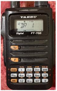
This radio (FT-70) is currently on memory channel 12 and has been labeled "DR 1" for our 146.940MHz repeater. It is on FM on the left side. On the right, we have enabled AMS by long pressing the AMS button.
