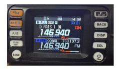
On an FTM-300, the channel is set to 146.940 repeater frequency setup with both DN and Tone Squelch PL Tone 107.2.
